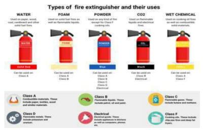
Fig. 9.7: Types of fire extinguishers
