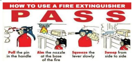
Fig. 9.8: Pass technique for Fire Extinguisher use
