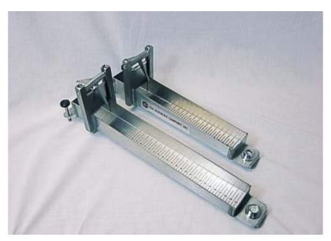
Fig 20.4 Bostwick Consistometer (Source: https://www.cscscientific.com/consistometer/bostwick-consistometer)
