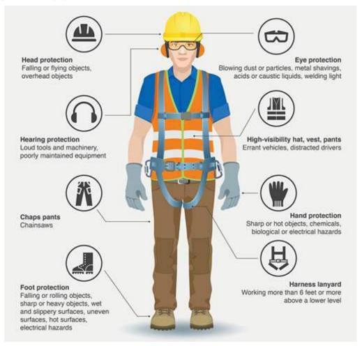
Fig. 9.5: The usage of personal protective equipment
